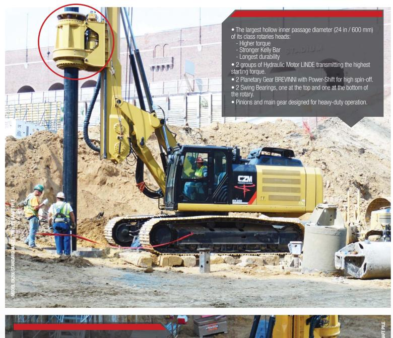
The mast is made of special steel called "Weldox" that has a yield strength 2,8 times higher than regular ASTM A36 steel. It means that with less weight the EK200 can have better stability and displacements on the job site and easier transport handlings
